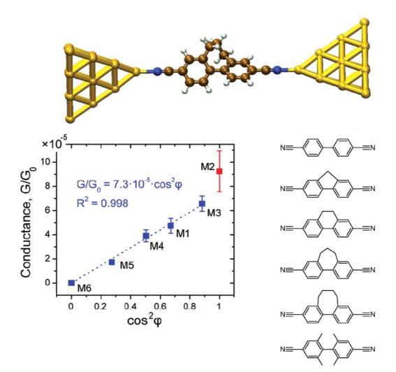
*Top: Metal – molecule – metal junction for one of the studied molecules. Lower left: Measured conductance vs cosine square of the torsion angle. Lower right: Analyzed molecules*
